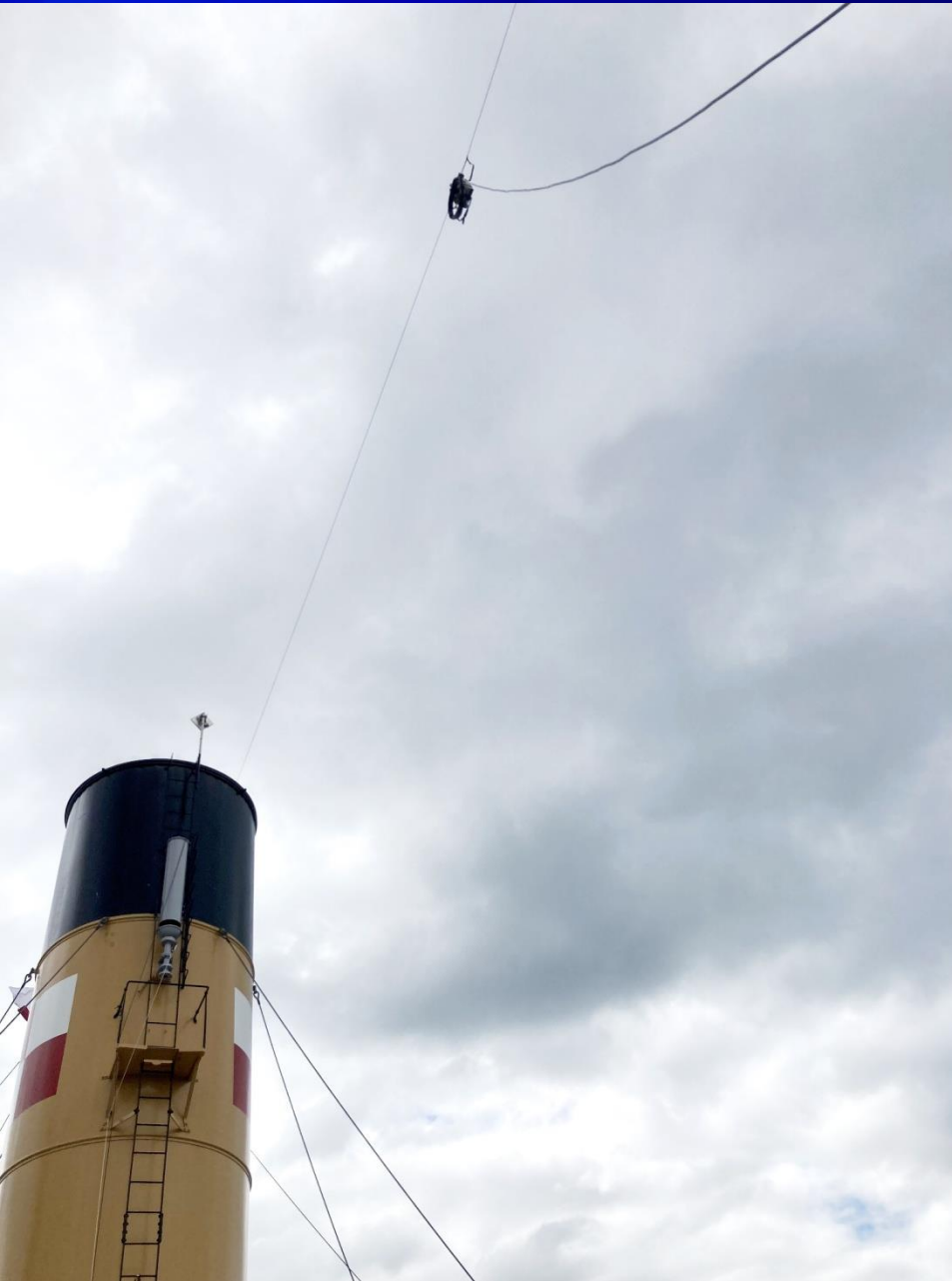
The HF antenna now in place between Keewatin's funnel and her forward mast
