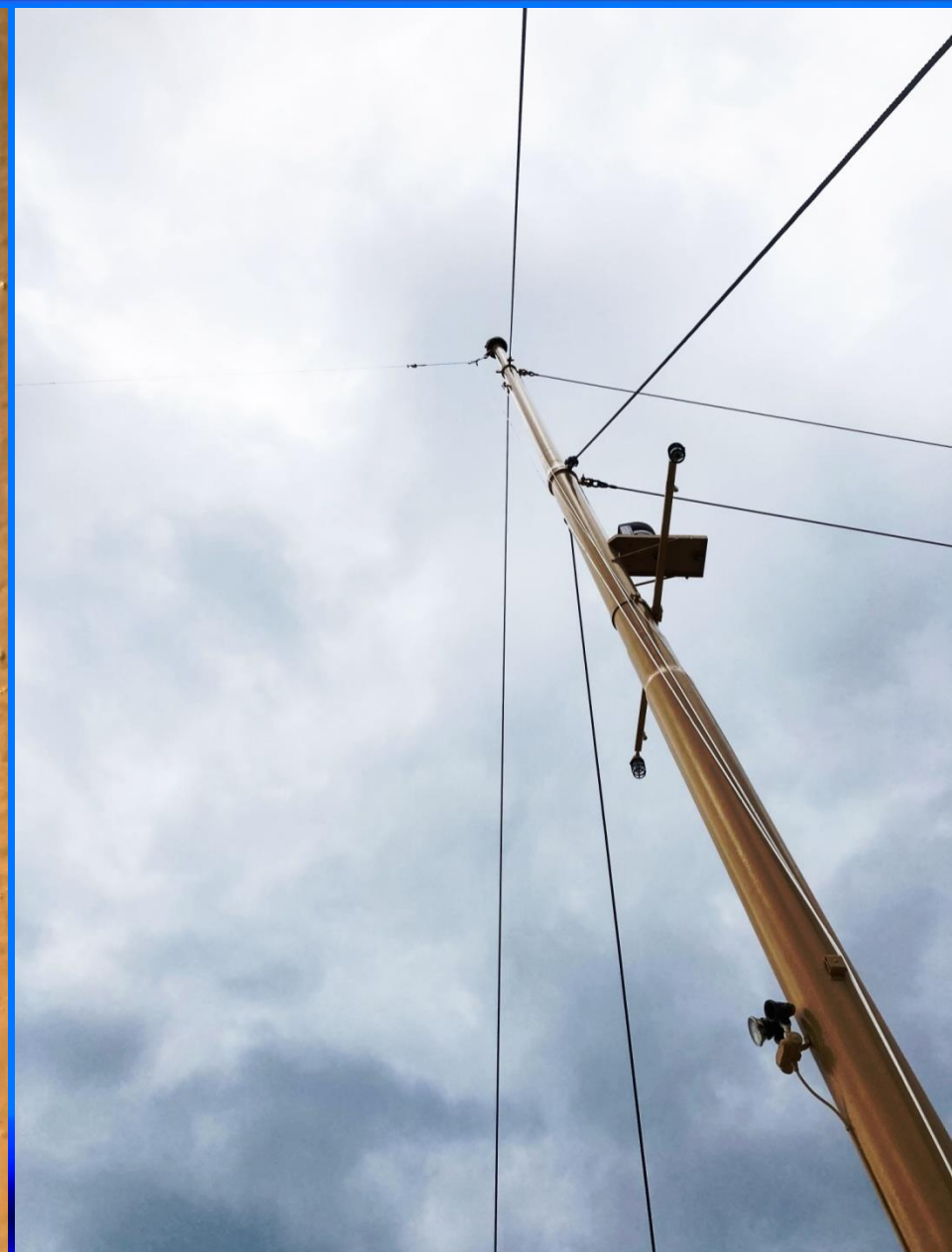
Hardware for the forward end of the HF antenna installed on Keewatin's forward mast
