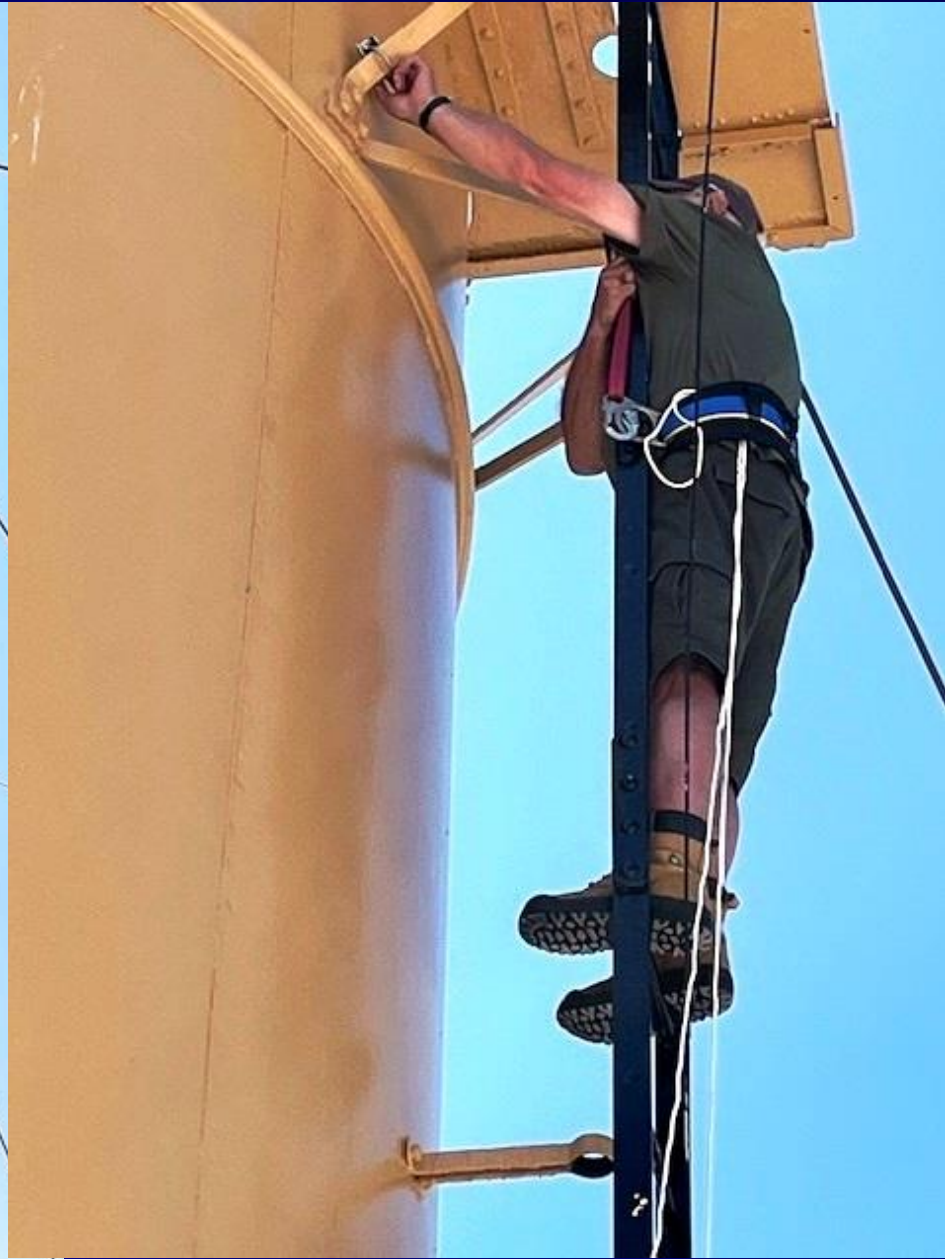
Hardware for the aft end of the HF antenna being installed on Keewatin's funnel
