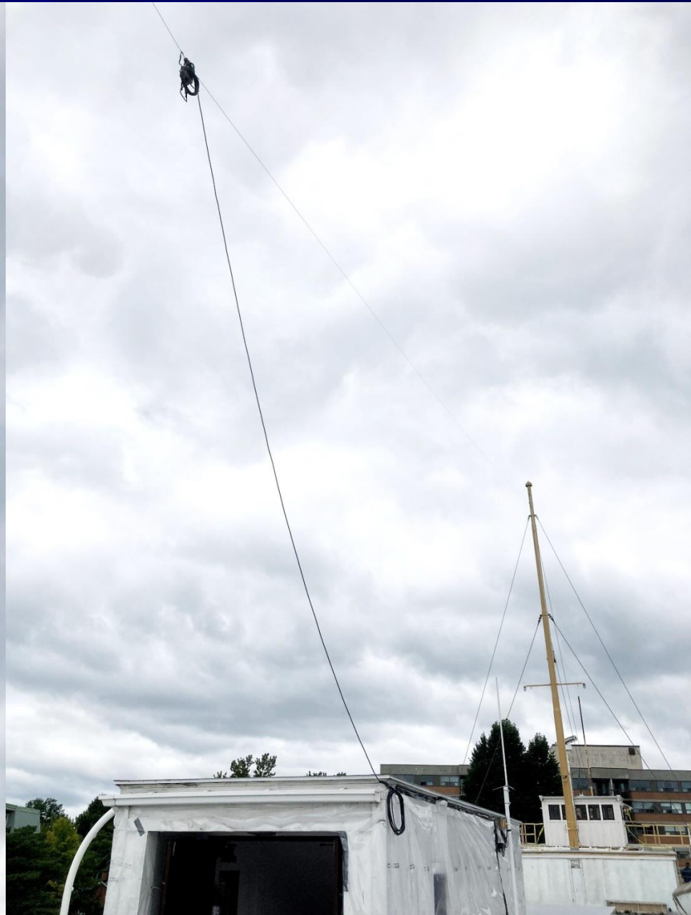
The HF antenna now in place between Keewatin's funnel and her forward mast
