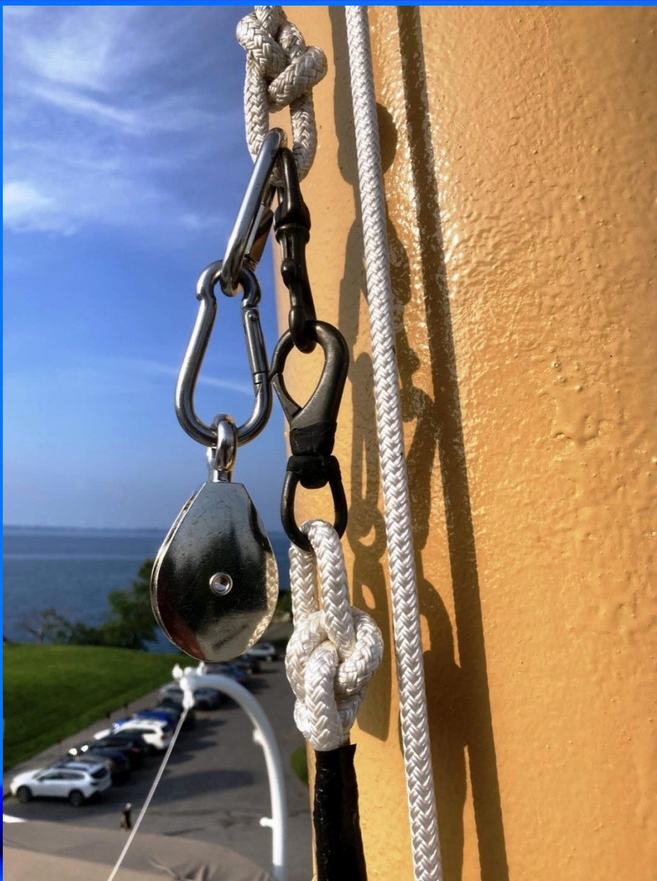
Hardware for the forward end of the HF antenna installed on Keewatin's forward mast
